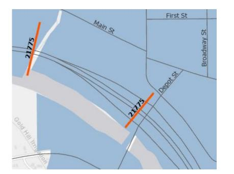
This project will widen the Evans Creek Bridge to the west side (Southbound lanes), widen the bridge over Depot Steet to the west side (Southbound Lanes), and remove portions of the bridge driving surfaces of both bridges as well as place new surface as well as replace the deck expansion joints.
