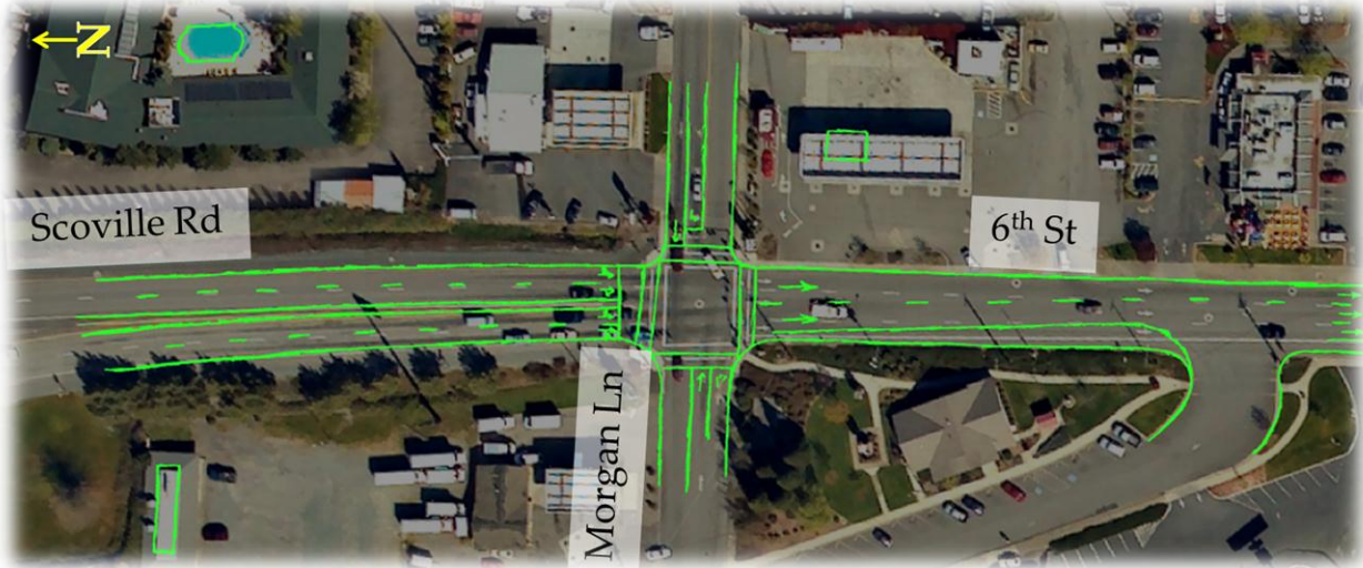
Exhibit 10 Downstream re-striping and relocated stop bar
