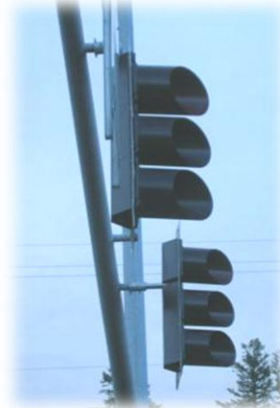
Exhibit 28 Example of extended signal head visors
